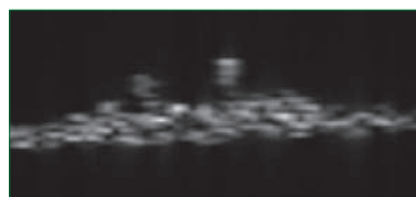
simulation of the roll, pitch and yaw allows Inverse Synthetic Aperture Radar target images to be produced.
